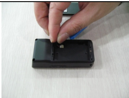
Figure 8 - Replacing KDC Battery
