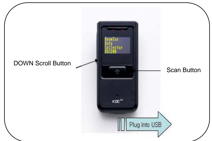
Figure 6 - Reset Function for KDC200 - KDC200P - KDC300
