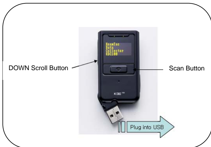
Figure 7 - Reset Function for KDC100
